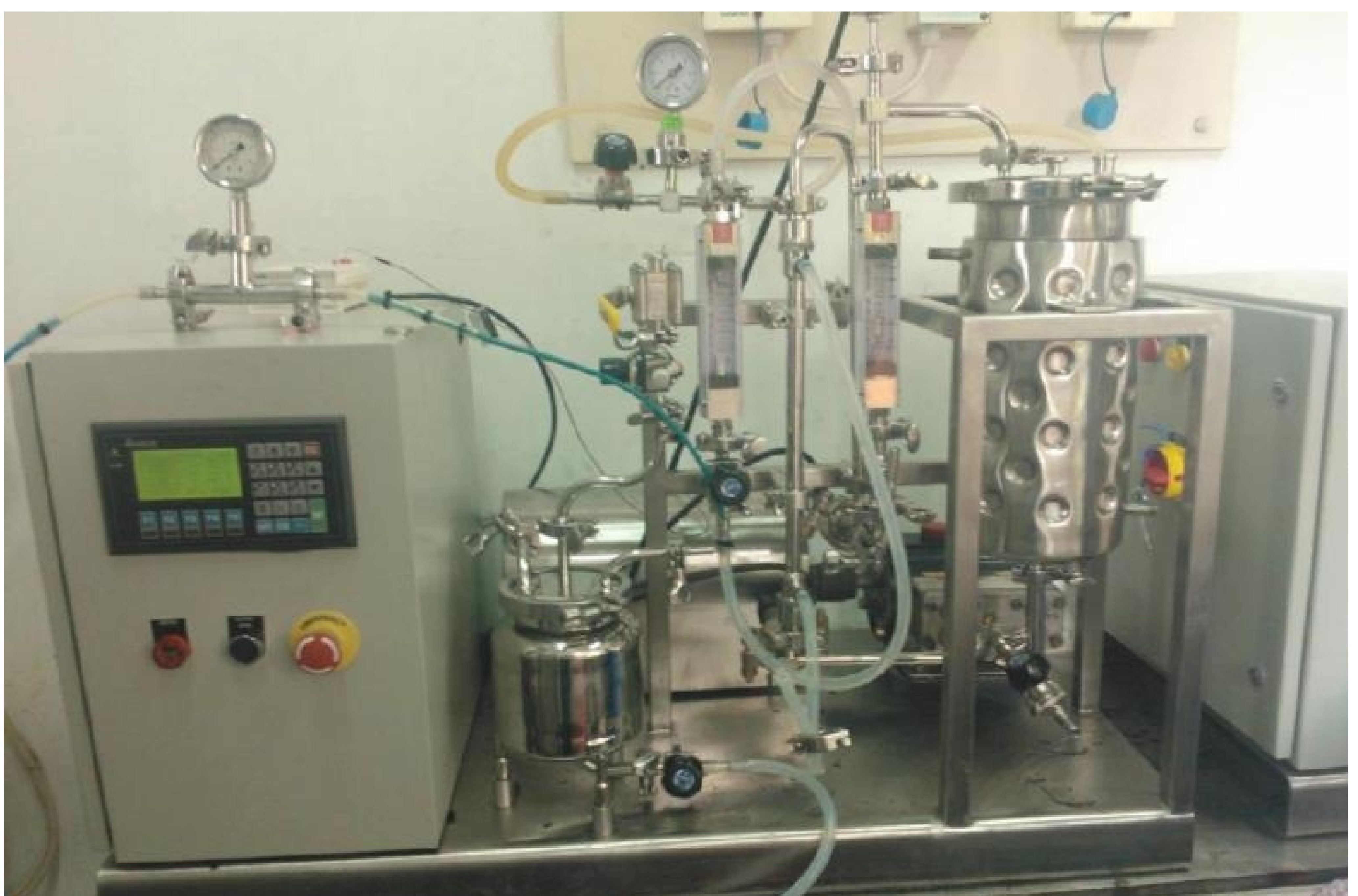
Bio-Catalytic Membrane Reactor
